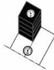
1.7 shared but separate electric meter
